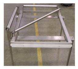
Allows web to make a 90 degree turn after it exits the splicer
